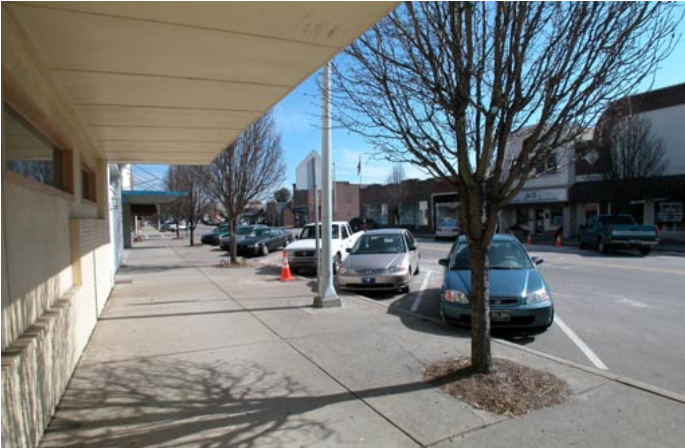
View of existing streetscape along the north side of East Montague Avenue in the historic commercial district. The lack of activity is accentuated by minimal windows or street furnishings. The street trees are not appropriate for this condition because they do not have a shade canopy.
