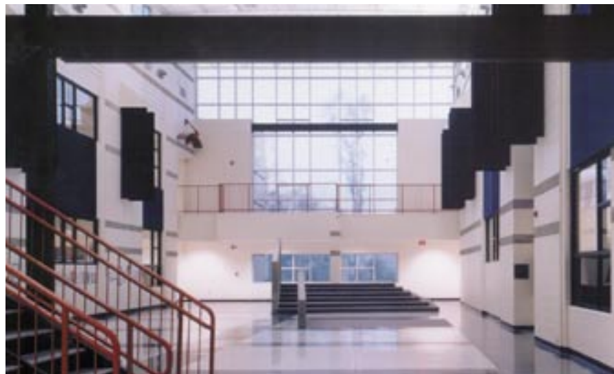
High quality daylight enters classrooms through windows and roof monitors. Combined with the light-colored interior finishes, this reduces the amount of energy expended to light each classroom.
