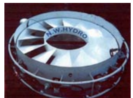
Innovations in hydro electric power include fish-friendly turbines developed for coastal and inland waterways
