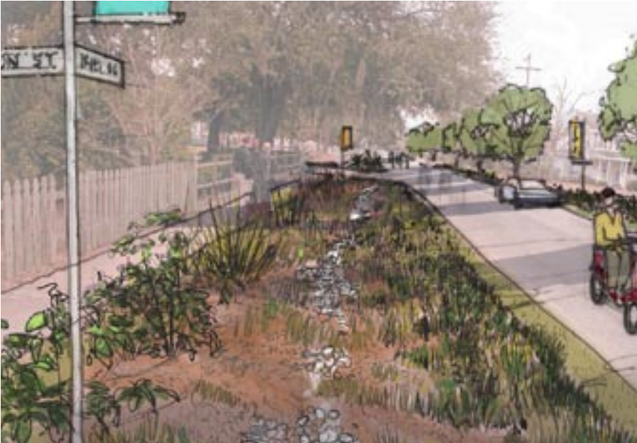
This section illustrates how streets could be modified to use a vegetated swale within the right of way.
