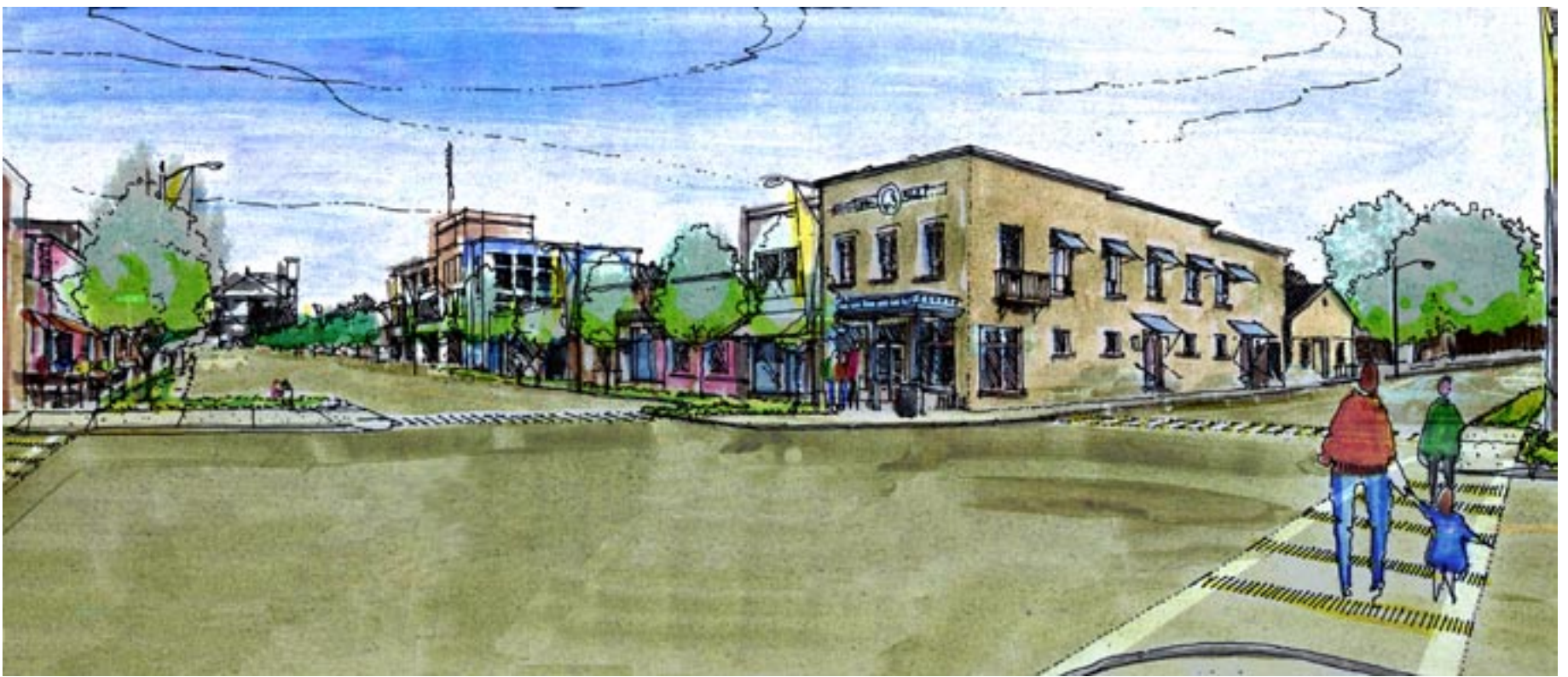
After - The proposed concept maintains the existing angled parking space in front of the commercial development. Additional landscaping and streetscape amenities are added. At each intersection the curbs are pulled out into the pavement, better delineating pedestrian paths and shortening distances traveled between curbs. Each intersection is further delineated with landscaping benches, and trash/ash receptacles. It is the hope that new commercial developments will infill Old Village.
