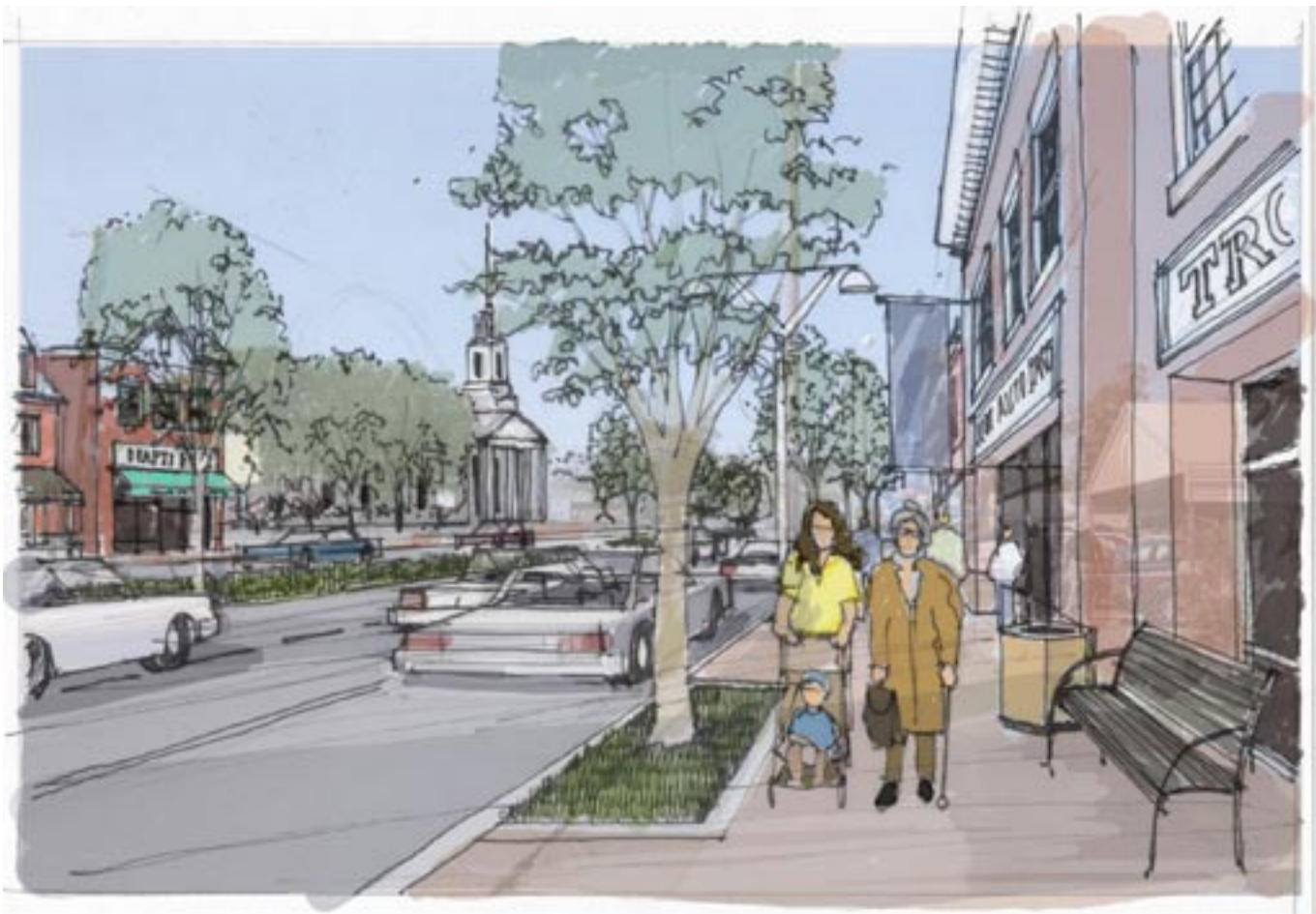
Encouraging infill development and decreasing the width of Rivers Avenue would help reduce the car-oriented scale back to a more desirable pedestrian scale. Landscaping the sidewalk and the new stormwater management swale at the median would make the area an attractive place for people again. Reorienting the street to the pedestrian will more strongly tie the Whipper Barony neighborhood back into the fabric of the Noisette area.
