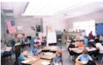
High quality daylight enters classrooms through windows and roof monitors. Combined with the light-colored interior finishes, this reduces the amount of energy expended to light each classroom.
