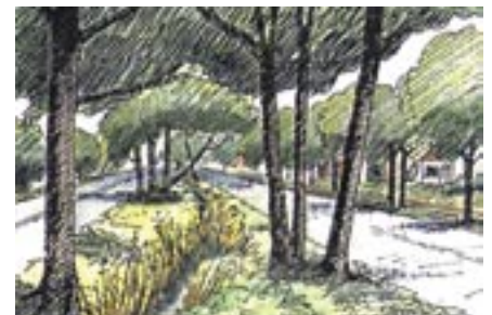
This is a graphic representation of what could replace the open ditch at Rivers Avenue. By using vegetated swales, with trees, grasses and sedges, surface runoff can be retained and cleansed before discharged into Filbin Creek.
